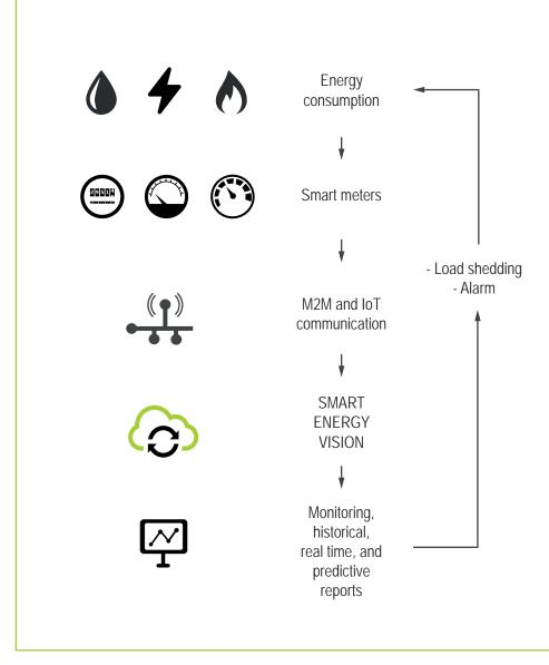
SMART ENERGY VISION is a platform for measuring real-time consumption data from virtually any type of energy meters, and even green energy generation. Local PLCs combined with Future Energy's advanced redundant OPC technology enable the collection of measurement data from the newest smart meters and older models, even in industrial, EMI-polluted environments.
